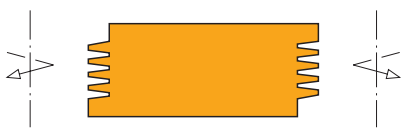
Profile 2 with staggered shoulder cutters
