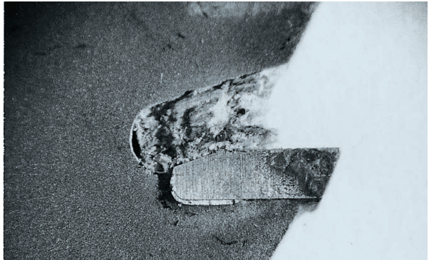
Cutting edge destruction through improper use.
