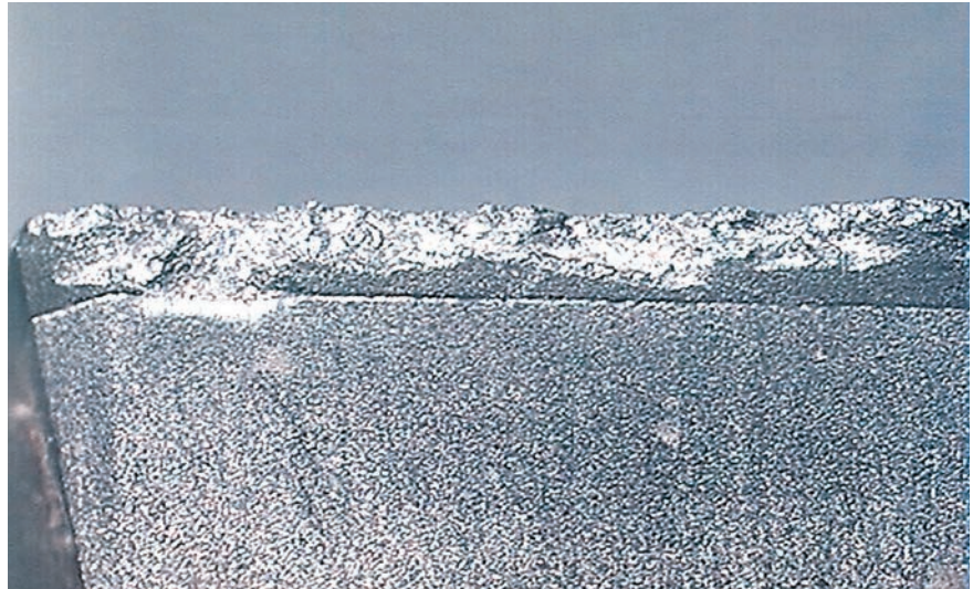
Cutting edge fracture of a DP saw tooth.
