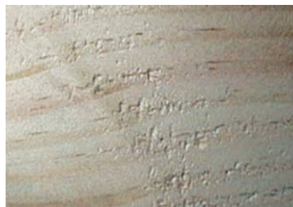
Finish planed surface after conventional preplaning.
