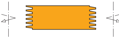
Profile 1 with continuous finger jointing
