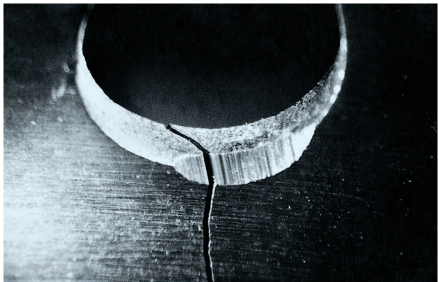
Fracture in the saw body.
