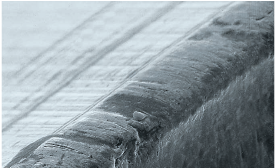
Wear of HS cutting edges.
