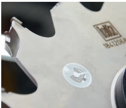
Tool with integrated NFC Chip
