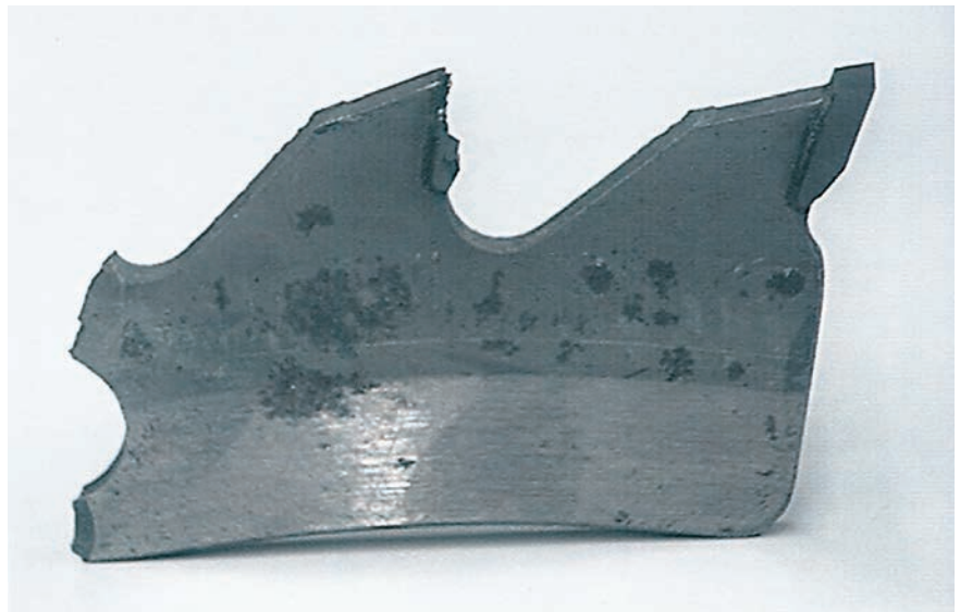
Destruction of saw tooth through overstress.
