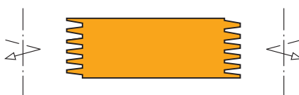
Profile 1 with continuous finger jointing
