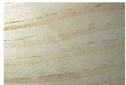
Finish planed surface after preplaning with RipTec.
